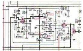
It is impossible to tune this transformer. I suspect the internal capacitor had changed his value due to chemical processes. It is the very same purple core device as in the TX chain. The solution is similar: add a capacitor between both 22 ohm resistors at the opposite end of the gate. Then it tunes flawlessly.
