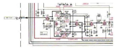
On the schematic diagram you can see **L45** and the built-in capacitor printed on the drawing without a value next to it. The cure is adding an external capacitor at this point.
