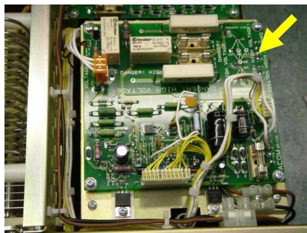
Fig.4 Mains PCB and voltage-selection jumpers location
