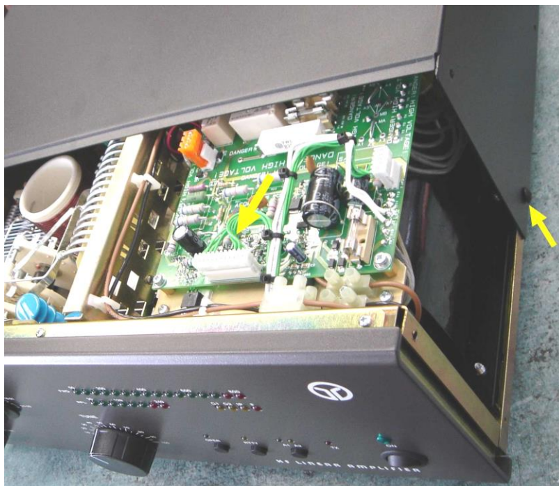
Fig.5 Top cover in service position
