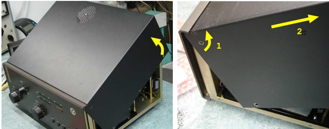
Fig.2 Top Cover Removal
