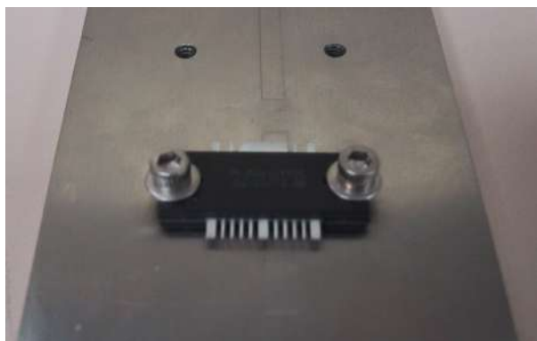
Figure 4. Simulated Bolting Down on Non-Flat Surface
