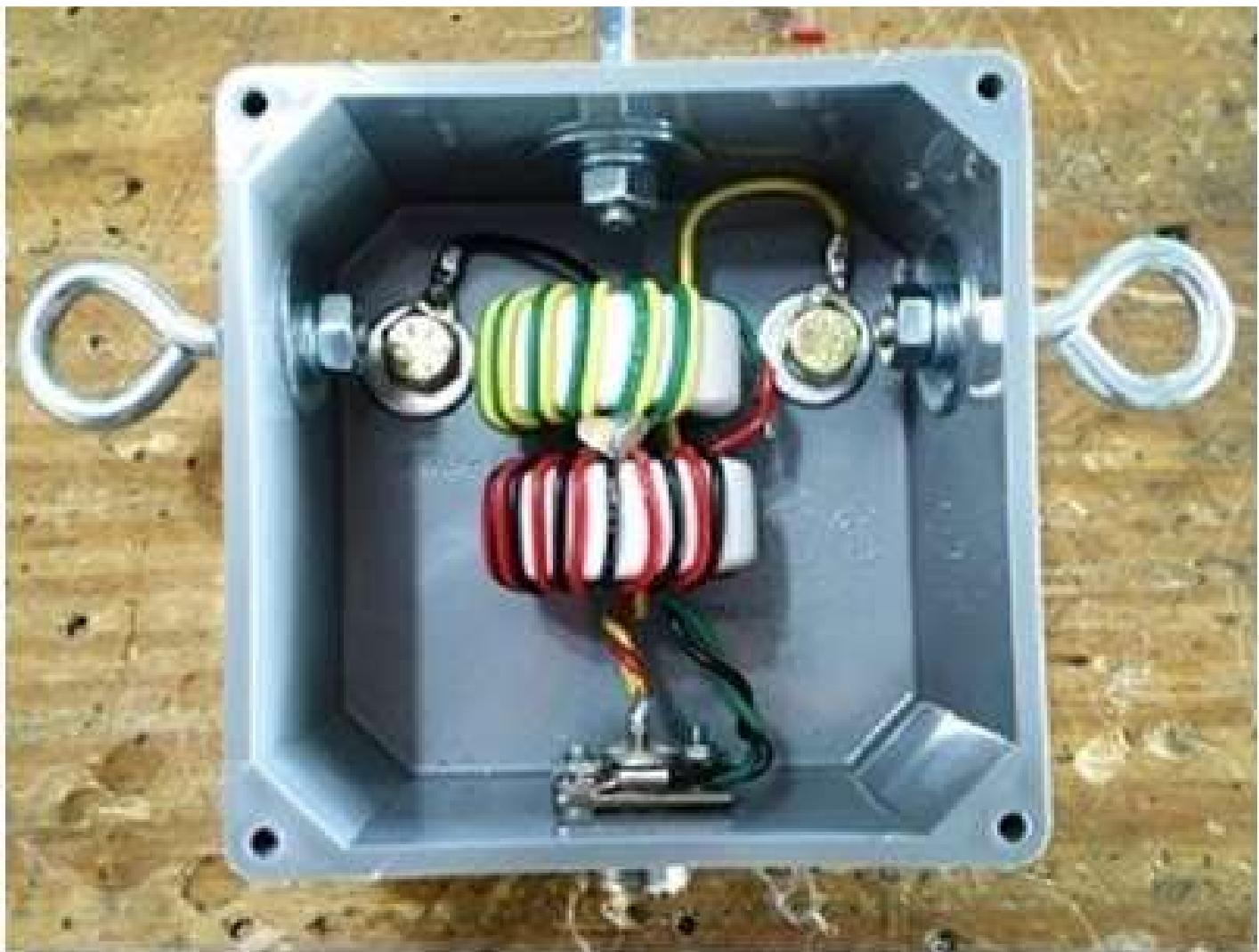
Connect 3 wires 3 and 7 to the SO-239 shield and wires 1 and 5 to the center conductor. Wires 2 and 8 connect to the large lugs for the dipole elements. Crimp and solder each connection. Keep the wires short but not tight. Route the wires clear of the case and metal edges. A small amount of RTV silicone or epoxy is needed to keep the cores secured in the wind. Less is better. DO NOT get any glue on the RF connections.
