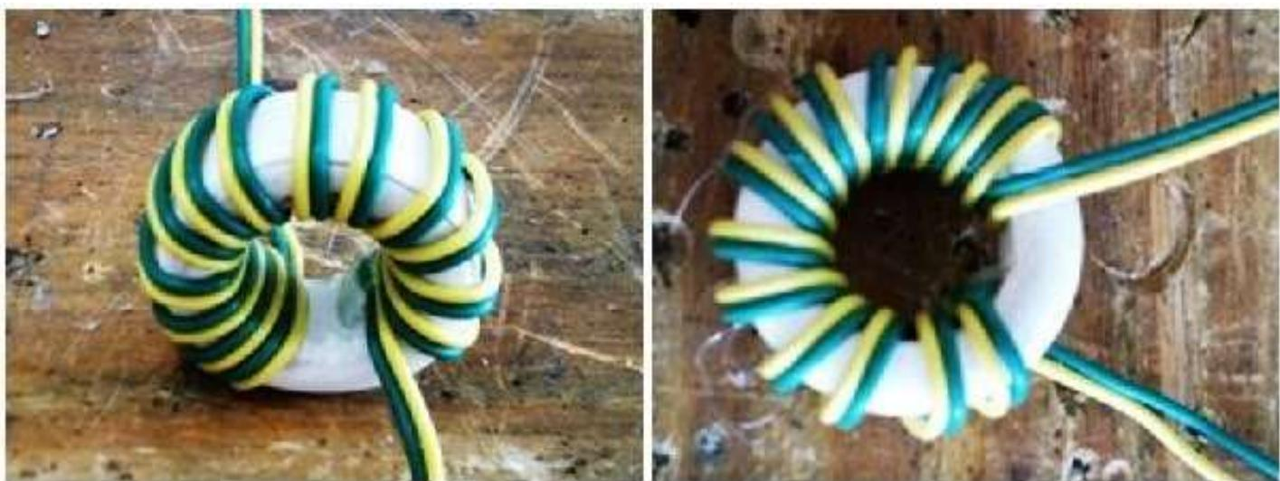
As shown above line up your wound cores in the same direction as the windings and label the wires to match the schematic below.
