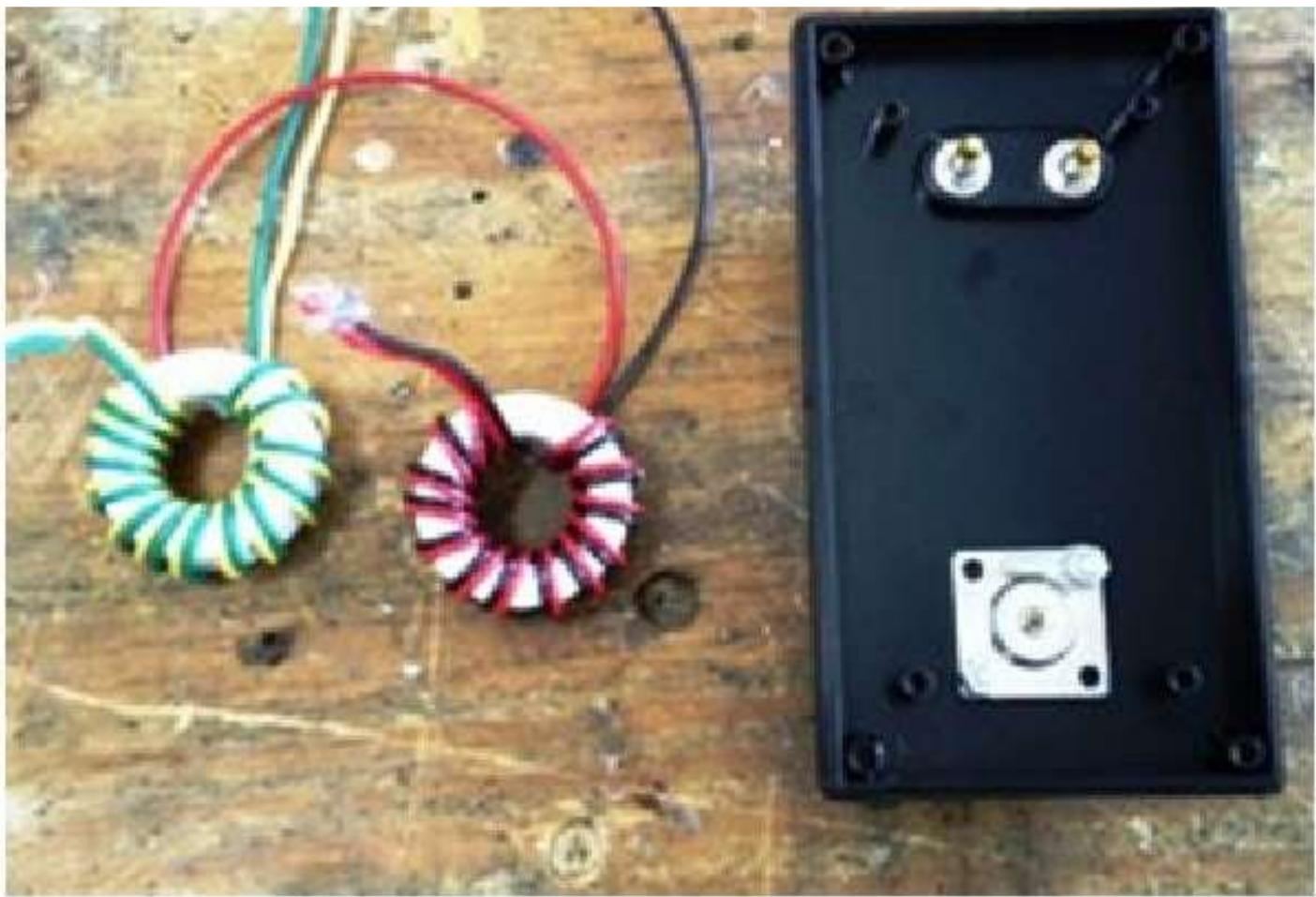
The cores, winding and wiring are the same but the box and antenna connection are different. The antenna is connected through a Panel Mount (red/black) Dual Binding Post commonly used on test equipment. The price is reasonable and the dielectric is 1000V rated.
