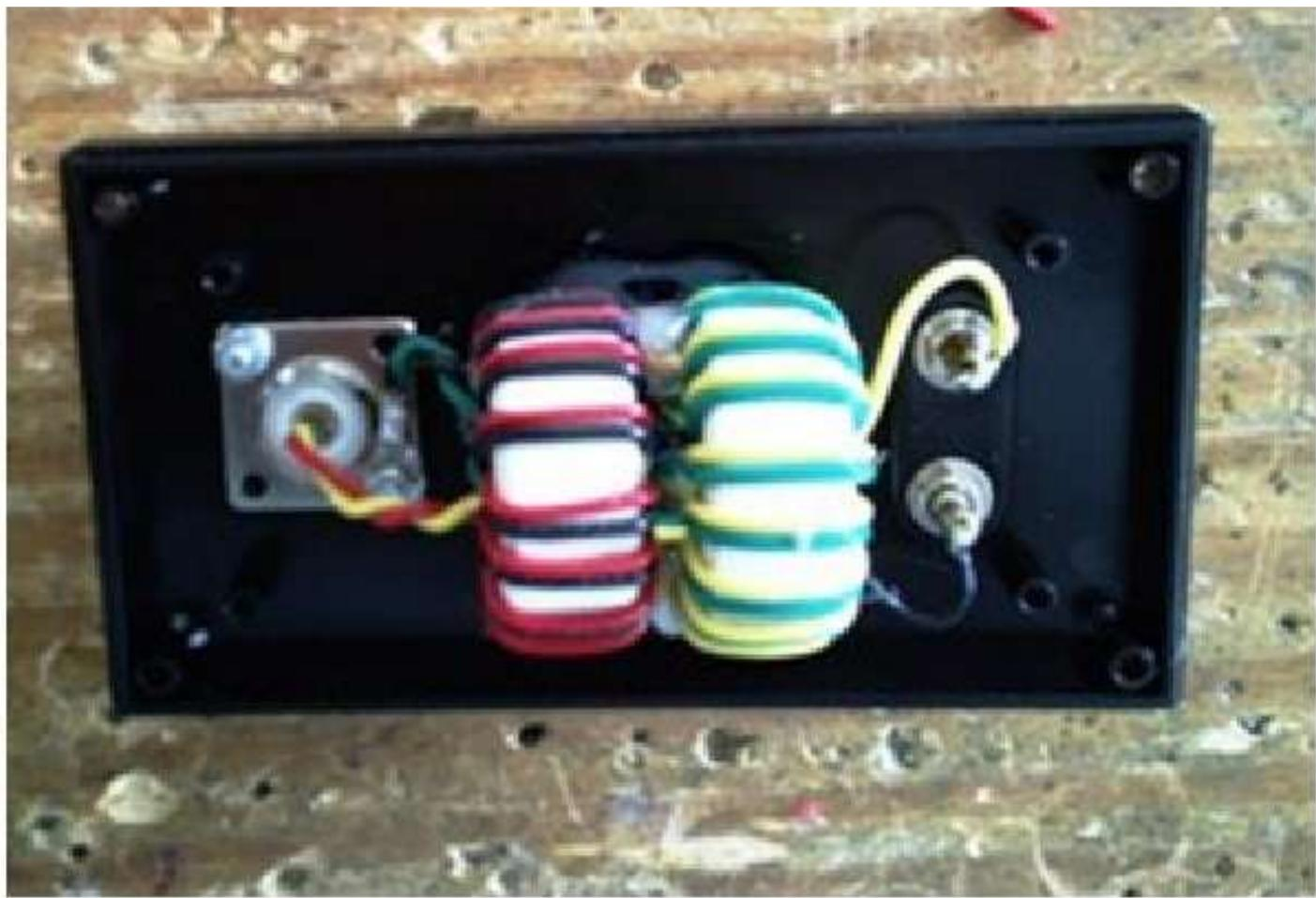
The box must be selected to fit the core size used for this case 6 X 3 X 2 Inches. Using the lid for all connections makes construction simpler by providing better access.
