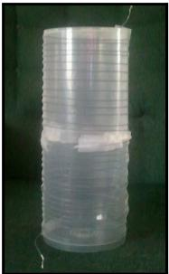
To use my short 20 Foot random wire on 160 meters, I add an extra coil, crudely wound on old plastic CD boxes, between the antenna wire and tuner output. The extra coil allows the tuner to provide a good match to the 20 foot wire on 160 meters. The Tuner, Coil, and 20 Foot Wre provides a very *inefficient* antenna on 160 meters, but it is *usable*. I only operate 160 meters during contests,
